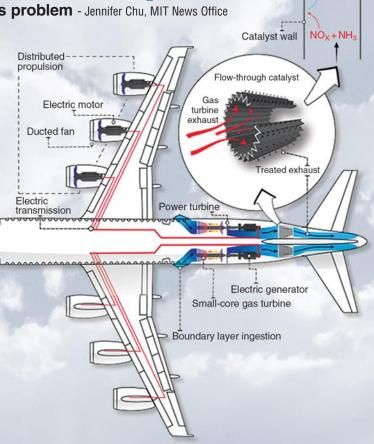
Barrett's concept gets around this limitation by separating power generation from thrust production, with exhaust from the gas turbine power unit fed into an emissions-control system, which could be folded up, accordion-style, in the plane's cargo hold. He envisions the bulk of the hybrid-electric system—gas turbine, electric generator and emissions control system—would fit in the belly of a plane, where there can be ample space in many commercial aircraft.
