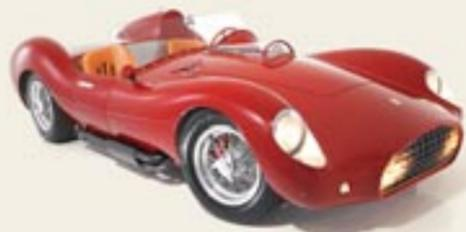
inspired performance BMW V12 with one-off cylinder heads, from the BMW factory in Germany and a custom Hilborn racing fuel injection system transmits power through a matching 6-speed transmission. Add tubular, adjustable suspension arms, BRT rack and pinion steering, racing-bred sway bars and many other competition tech advancements, plus Brembo and Wilwood racing disc brakes.
