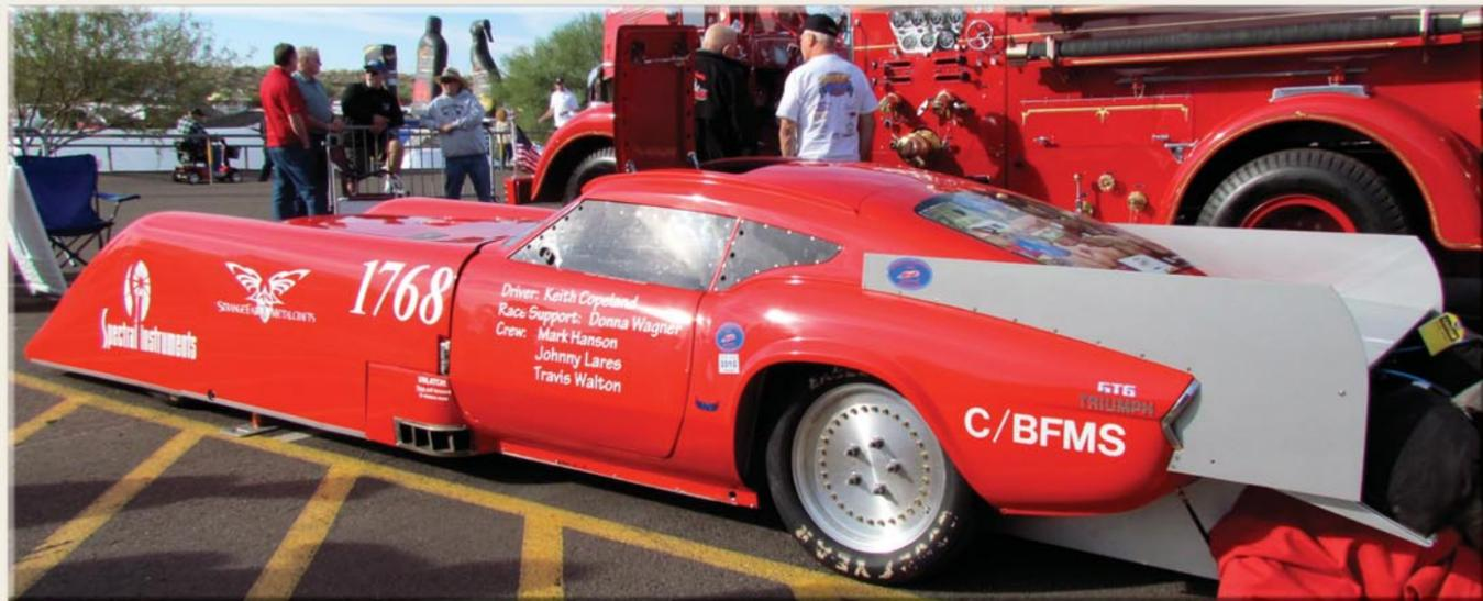
For one thing, the wheelbase was stretched from 83 to 130 inches. For another, a 360-cubic-inch Brodix-block V8 engine was installed, and topped with a pair of turbochargers. Power—1400 horsepower—from that engine goes to the front wheels, not those at the rear.
