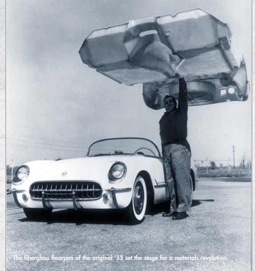
The fiberglass floorpan of the original '53 set the stage for a materials revolution.
