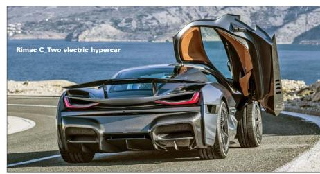
active height adjustment create a smooth and comfortable ride, while four electric motors, one powering each individual wheel, provide both four-wheel drive and extremely high levels of dynamic control. A pair of independent single-speed gear-boxes applying drive to the front wheels, plus a pair of independent two-speed, gearboxes, one for each rear wheel, allow the C\_Two to make use of its prodigious
