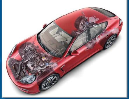
Vectoring Plus, using braking force to control speed and yaw rate in cornering.
