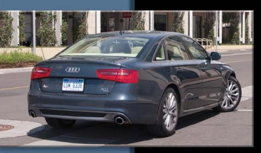
of this, but the wind tunnel also comes into play: the new body reduces drag coefficient by over ten percent, from 0.29 in 2011 to 0.26 in 2012. Efforts didn't stop with the wind tunnel. The new
