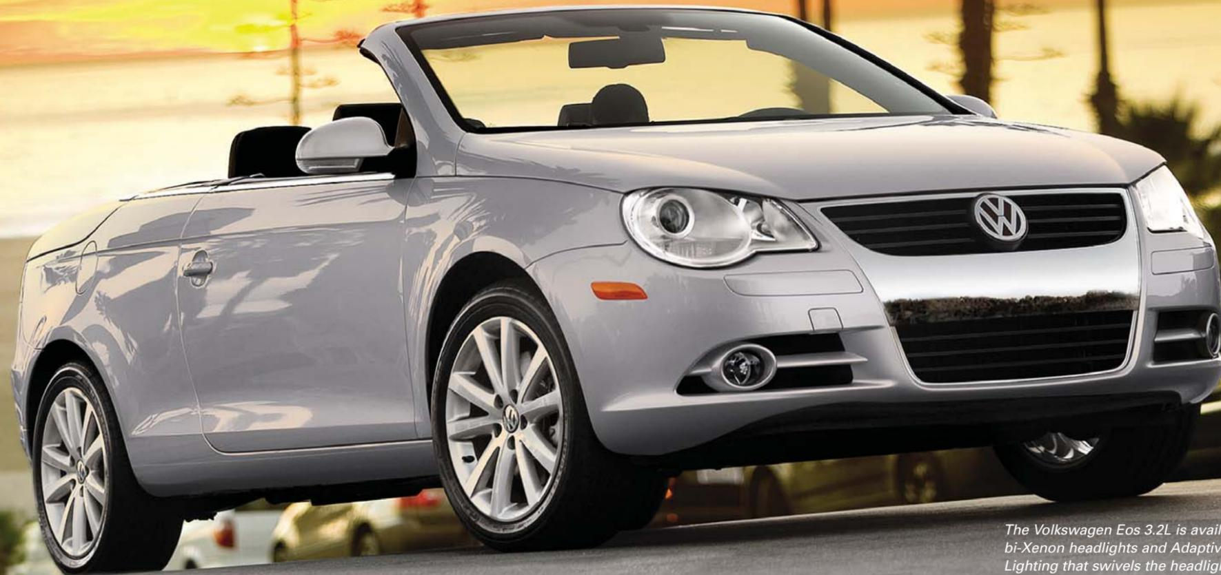
The Volkswagen Eos 3.2L is available with bi-Xenon headlights and Adaptive Front Lighting that swivels the headlights horizontally at highway speeds to improve nighttime vision around curves.
