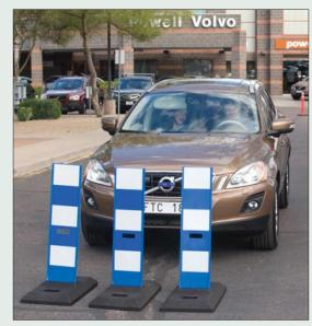
We tried the City Safety System at Powell Volvo on McDowell Road in Scottsdale. Instead of the inflatable car Bill and Barbara tested with, we had three vertical barriers. It can be disquieting (not surprisingly) to bear down on an obstacle with no intent to brake, but not as disquieting as the crash you could one day have without this feature. Volvo points out that this system applies 100% of the brakes, compared with about 40% maximum by most humans.
