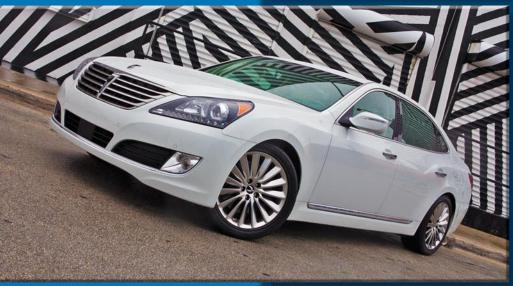
he 2014 Equus is a mid-cycle refresh. Up front are a revised grille and fascia, while LED foglights have been added and superfluous chrome accents have been removed. Side mirrors have been restyled for better aerodynamics and a quieter ride, and new 19-inch wheels feature a distinctive turbine blade design. In back, there is another reduction in chrome, and LED taillamps are restyled. Rectilinear dual exhaust emphasizes the car's confident stance.
