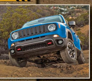
inches or articulation, with 8.7 inches of ground clearance (which matches Cherokee). Sport, Latitude and Limited models have slightly lower clearance, more geared toward highway travel or more moderate outings. (More drivetrain and suspension details are given in photo captions.)
