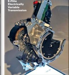
A core component of the Chrysler Pacifica Hybrid's eHybrid system is its E-Flite Electrically Variable Transmission (above), an in-house development which operates in both electric vehicle (EV) or hybrid electric vehicle (HEV) modes, utilizing two electric machines and planetary gear set with oneway clutch. The innovative one-way clutch enables both electric machines to drive the front wheels in electric-only mode.
