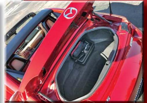
Some retractable hardtops gobble up the entire trunk when the top is down. Some just part of it. The new #Mazda MX-5 #Miata RF's top does not take up any at all. (There's a difference of 11/100ths of a cubic foot, same up or down, presumably from a tiny volume for a motor or strut or something... totally negligible.)
