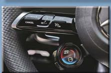
One style-over-engineering trend we would send back for further development are the shiny black membranes covering switches for many key functions. There is little or nothing to distinguish, by touch, what could be buttons, necessitating eyesoff-road at critical times. Even when parked and
